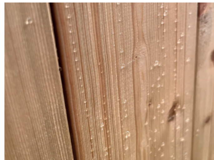
Water beading and run off after oil treatment
