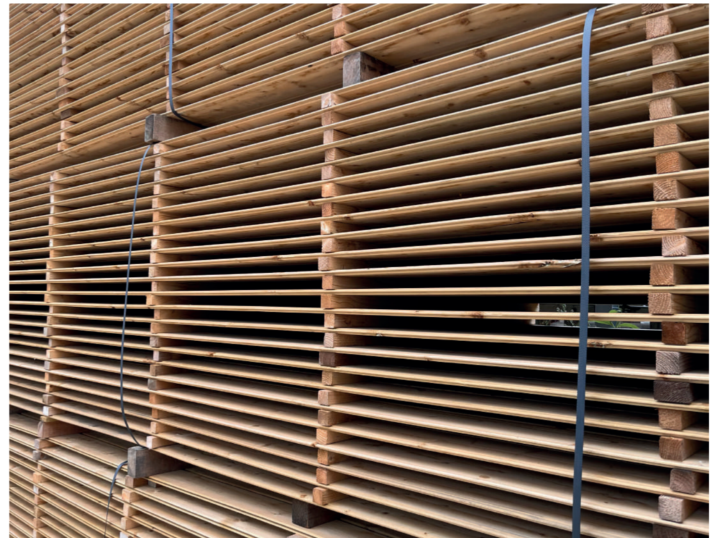
Latted timber drying process
